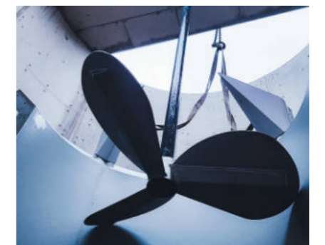
Mixing Reactor System – effective interaction with a fine-bubble ventilation
